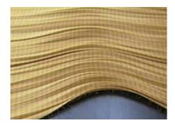
The terminology "synthetic tire cord layer" used in this part of ISO 17357 refers to tire cord made of synthetic fibers. Synthetic tire cord layers, commonly used in tires, have been proven to provide strong efficient reinforcement layers in fenders. Each single layer is coated with rubber compound on both sides as well as in between synthetic tire cord threads, hence isolating all cords from each other.
